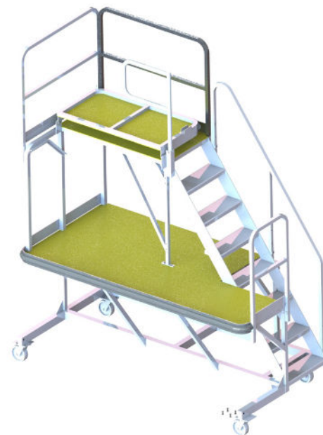
UPPER ACCESS PLATFORM IN FOLDED POSITION
