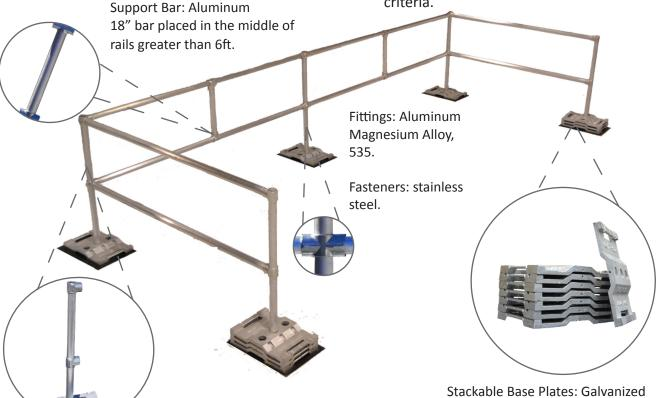
Pipe: Aluminum T6-6061, 1.5" SCH. 1.90 inches O D. stackable Base Plates: Galvanized cast steel weights (40 lbs) with three optional holes for vertical post-placement. Includes handles to avoid pinch points. Masticated rubber pad included.
