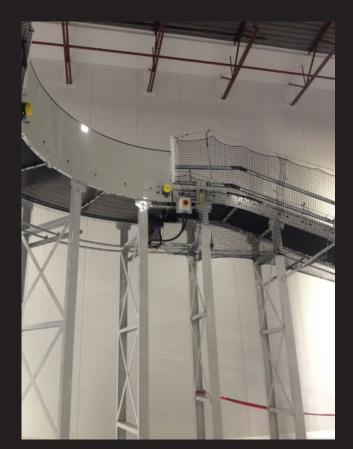
Protect employees by installing conveyor netting systems to catch product from falling to the ground below.
