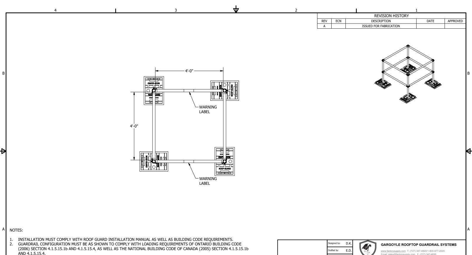
FOR A CUSTOM ENGINEERED SOLUTION TO MEET THE REQUIREMENTS. 4. NO MODIFICATIONS SHALL BE MADE TO THE SYSTEM WITHOUT PERMISSION IN WRITING FROM ROOF GUARD AND THE ENGINEER. ALL SET SCREWS TO BE TORQUED TO 13 FT-LBS.
